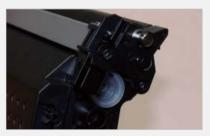
Install the E-Ring on the developer roller shaft.
