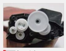
Remove the 5 gears.
