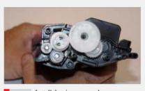
Install the six gears as shown.
