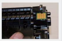
If available, replace the chip on the cartridge. (The chip can be re-used)
