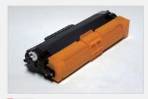
Wipe the cartridge down to remove any remaining toner dust.
