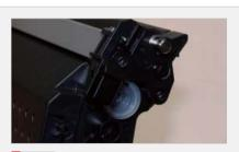
Remove the E-Ring and developer roller.
