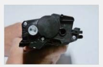
Install the larger gear side end cap, and three screws.
