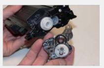
On the non-gear side of the developer roller remove the 2 screws and remove the end cap.
