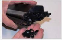
Pry up the tab and remove the inner end cap.
