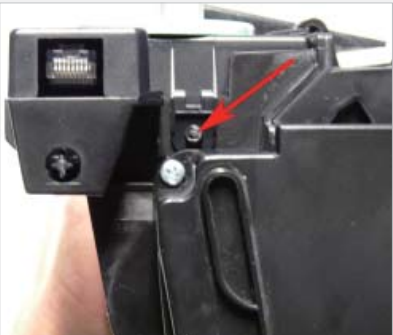
STEP > 14 Press the chip housing back in place. Make sure the three tabs are locked and the cover is fitting properly around the alignment tab.
