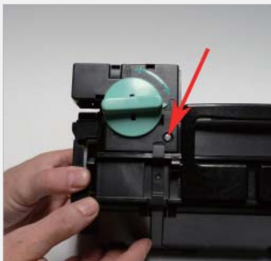
step > 8 Remove the screw located next to the large green knob.
