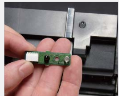
step > 12 On the opposite end of the wires is a toner sensor board. Shown here just for information purposes. There is no need to remove it.
