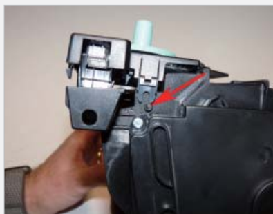
step > 9 Press in on the three tabs to loosen the cover. Be careful not to break the alignment tab.
