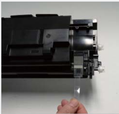
step > 6 Clean the port seals and install a new seal. (You can make one from clear tape folded back on itself until one is available).
