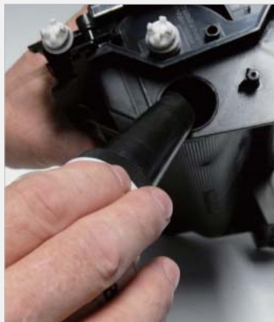
STEP > 16 Fill the hopper with the appropriate amount of toner for use in the ProXpress SL-M4530 series of cartridges.
