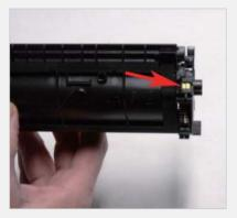
Check to make sure the spring loaded arm moves freely.
