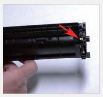
Replace the chip by pressing down on the locking tabs and sliding the chip out.
