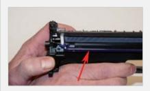
If any toner got onto the blue doctor blade seal, clean it with isopropyl alcohol and a foam swab. We do not recommend using a cotton type swab as they can leave threads of cotton behind which can cause a leak.
