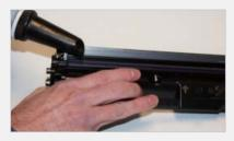
Fill the cartridge with toner approved for use in the HP LaserJet Pro M118 series of printers.
