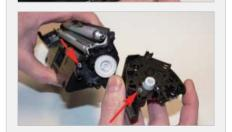
Press in on the bottom tab and carefully pry off the end cap. Work the end cap from multiple sides, there is a plastic post that must snap before the end cap will come off.
