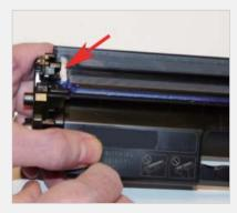
Clean out any remaining toner from the supply chamber. Be careful to clean developer roller seals.
