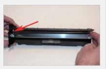
Insert the magnet into the slotted bushing on the left side of the cartridge. Be careful to align it properly, forcing the magnet in will break the bushing.
