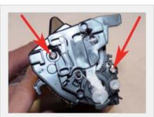
Place the cartridge with the handle facing up. Remove the two screws on the right side end cap. Both of these screws have a left hand thread.
