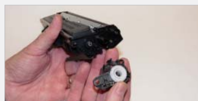
step > 8 On the reset gear side of the developer roller remove the 2 screws and remove the end cap. Note that the reset gear stays with the end cap!
