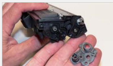
step > 9 Remove the black inner end cap.
