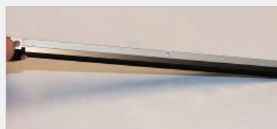
step > 14 Vacuum the doctor blade clean. The doctor blade can be easily cleaned by blowing the excess toner off, and wiping down with a lint free cloth. Be very careful not to leave any lint behind!
