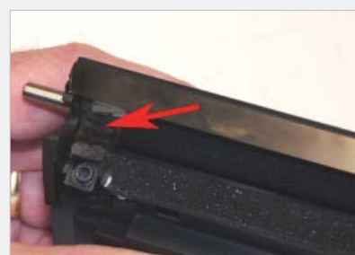
step > 15 Inspect the developer roller felts. If they are compressed, (shiny) rough them up with a small screwdriver.
