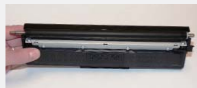
step > 19 Re-install the developer roller with the long shaft to the gear side.
