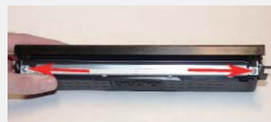
step > 18 Install the Doctor Blade and two screws.
