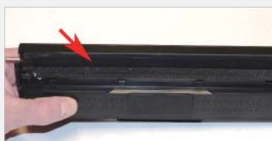
step > 13 Clean out any remaining toner from the hopper. Pay special attention to the feed roller to make sure it's clean.
