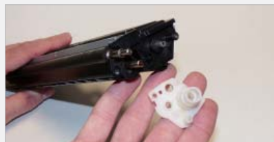
step > 7 Remove the white inner end cap.
