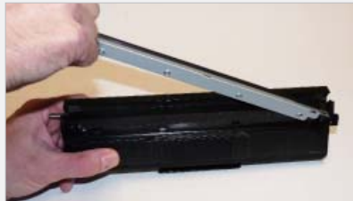
step > 12 Remove the two screws and Doctor Blade. Be careful not to damage the foam DB seal while cleaning.
