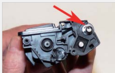
step > 10 Remove the E ring from the developer roller shaft.
