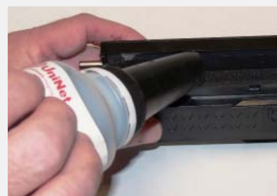
step > 17 Fill the cartridge with toner for use in the Brother HL-L3290 series of toner cartridges. Make sure you use the correct color for your cartridge.
