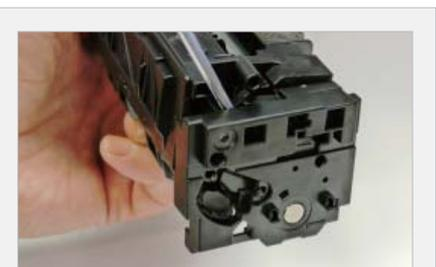
**3** Slide the screwdriver inside the end cap to the place indicated and gently pry again until the end cap comes free.
