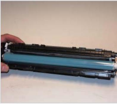
**29** Coat the drum with your preferred lubricant and install the drum in the waste hopper.
