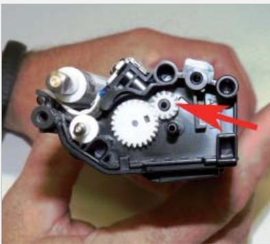
**step >** **22** Install the small and large gears as shown.
