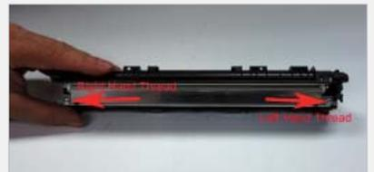
**step >** **20** Clean the doctor blade seals. Install the doctor blade and two screws. Remember the right side uses the left hand threaded screw! Make sure you have an even gap across the DB edge. They is not an alignment pin for the blade.
