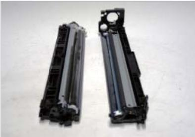
**step >** **6** Start to separate the two halves. You will see a small black plastic tab on the drum gear Assembly that blocks you from removing the waste chamber. Press down opposite the tab while pulling the end cap out to separate the two halves.
