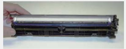
**step >** **18** Vacuum out the remaining toner from the hopper from the slot next to the feed roller. Remove the old seal if present.
