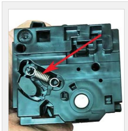
**1** With the HP top label facing you, remove the spring from the left side of the cartridge.
