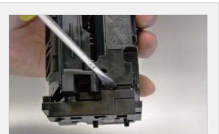
**2** On the same side, using a flat blade screwdriver, pry out the top of the end cap until you feel the weld give way.
