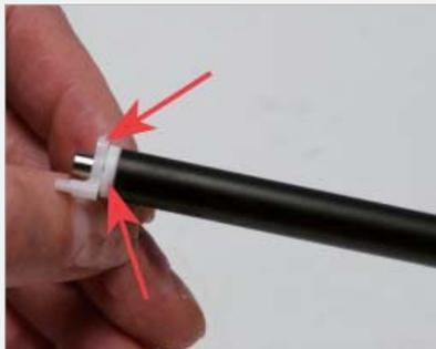
**step >** **16** Slide the developer roller over and remove. Be careful not to lose the 2 round bushings or alignment tab.
