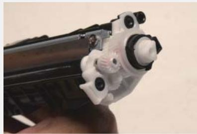
**step >** **25** Install the drum drive gear and bushing.
