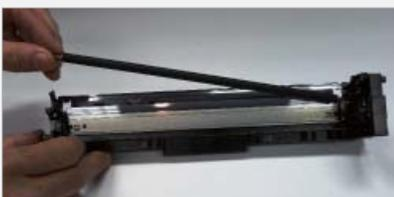
**step >** **7** Remove the PCR. Clean with your preferred PCR cleaner and place aside in a clean area.
