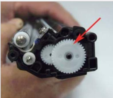
**step >** **22** Install the small and large gears as shown.
