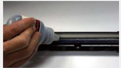
**step >** **19** At this point you can fill the hopper with toner for use in the HP M254 series of printers.
