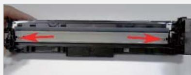
**step >** **10** Coat the new wiper blade with your preferred lubricant and install. Install the two screws.
