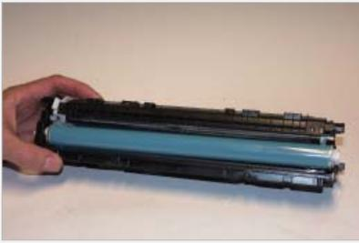
**step >** **5** Remove the drum from the cartridge. Doing this now will make separating the two halves easier.
