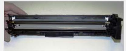
**step >** **11** Install the cleaned PCR. Make sure to place a small amount of conductive grease on the black PCR holder.
