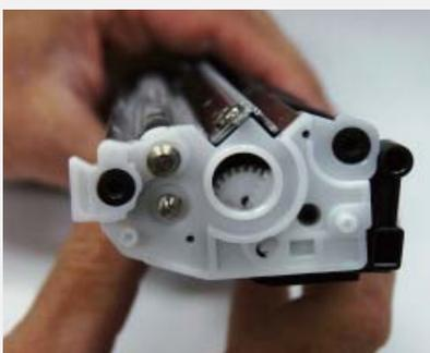
**step >** **23** Press the inner end cap in place.
