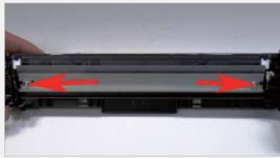
**step >** **8** Remove the two wiper blade screws and the wiper blade.
