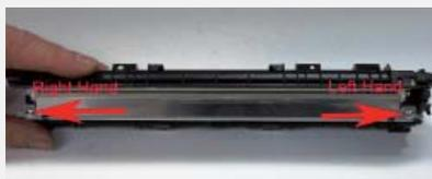
**step >** **17** There are two screws holding the doctor blade in place. The left screw is a normal thread screw, the right side uses a left hand thread screw. Be careful not to mix them up. Remove the DB.
