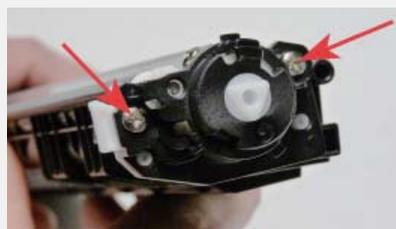
**step >** **26** Install the end cap and two screws.
