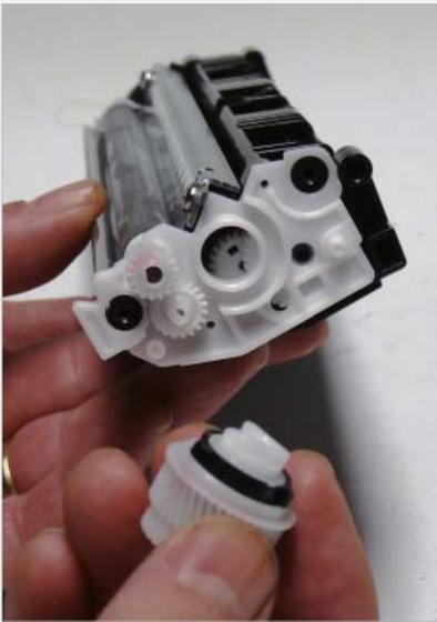
**step >** **12** On the Supply chamber, remove the two screws from the gear side end cap. Remove the end cap. Be careful of the drum drive gear and bushing. They can come loose.
