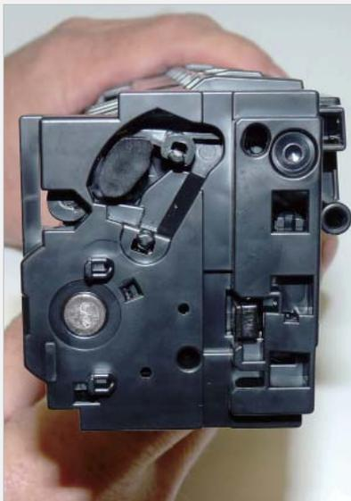
**30** Place a small piece of a good double-sided tape on the inside of the end cap. Clean and replace the conductive grease on the drum axle and install the end cap.
