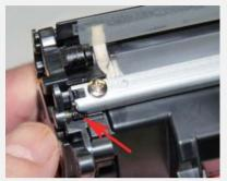
Re-install the doctor Blade and two screws. Make sure the contact sprint is touching the blade! This is a new type of contact for HP to use on this blade.
