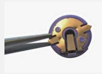
Straighten out the contacts on the contact gear.
