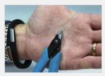
Grab the pins with a pair of pointed flush cutting wire cutters, and remove. Flush cutting wire cutters have blades that are flat on the bottom side. Normal wire cutters have curved blades. The flush cutting kind are better for grabbing recessed pins. Note that the pins for both sides are the same.
