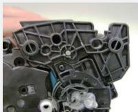
Place the two halves together, make sure that the two springs are aligned, and insert the two pins. Make sure that the pins are slightly pushed in so that they do not interfere with installing the cartridge in the printer.
