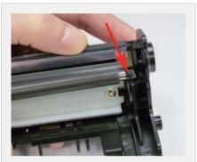
Re-install the cleaned PCR. Note that a new OEM PCR has a small amount of conductive grease on the black (contact) side.
