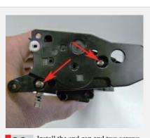
Install the end cap and two screws.
