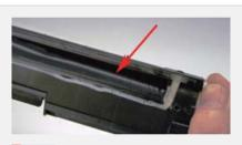
Remove the remnants of the old seal. These cartridges use a self-removing seal system. This picture shows a new cartridge with the seal starting to remove from right to left.
