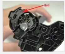
The drum hub on the opposite side is welded. The weld can be broken or drilled out, but there is a good chance that the hub will either warp if pried off, or will be hard to align if drilled out.
