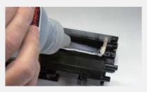
Fill through the Mag roller opening with \*g of toner for use in the HP CF226A or X series toner cartridges. There is not a fill plug in these cartridges.
