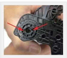
With a flat head screwdriver, press the drum axle pin out from the inside of the cartridge wall as shown. There is NOT a small shoulder as in older versions. Press the axle out just enough so that you can grab it with the flush cutting wire cutters. You may have to make two small cuts on each dies of the pin from the outside in order for the cutters to be able to grab it.
