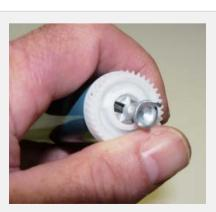
Install the drive gear. Place the drum onto a flat surface and gently tap the gear with a rubber mallet until the gears sits flush. (Do not hit the dongle gear!)
