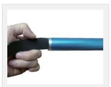
Lightly sand the inside of the new drum where you will be installing the contact gear. This will help ensure good electrical contact.
