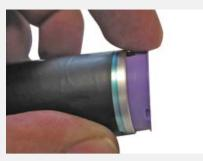
Apply a few drops of super glue around the inside of the new drum about 1/8" in from the edge. Make sure you leave space with no glue present for the contacts to touch the metal drum wall. These contacts must be metal to metal with no glue in between them. If any glue is in between the contacts and drum wall, there will be drum ground issues (solid black pages). Install the contact gear.
