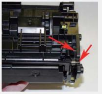
Install the drum cover; make sure the spring is situated correctly, and the slot on the cover fits into the tab on the cartridge.
