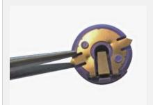
Straighten out the contacts on the contact gear.
