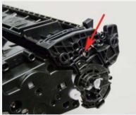
Place the two halves together, make sure that the two springs are aligned, and insert the two pins. Make sure that the pins are slightly pushed in so that they do not interfere with installing the cartridge in the printer.
