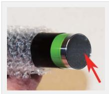
On the opposite side, place a few drops of medium or thick super glue on the inside wall of the drum about 1/8"in from the edge. This will prevent the glue from overflowing into the drum coating when the drive gear is installed.
