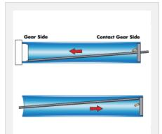
Slide a 1/16" metal rod about 18" long along the drum wall until it meets the side wall of the dongle gear. Lightly tap the rod a few times with a hammer, rotate the drum, do the same until it comes loose. Normally it will take three to four taps for the gear to come loose. Do the same for the contact side taking care not to place the rod anywhere near the copper contacts that bite into the drum.
