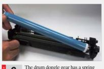
The drum dongle gear has a spring that holds it off to one side. (Necessary for it to engage the printer). Release the tail of the spring off the gear and remove the drum.
