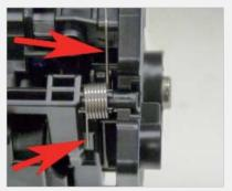
Remove the drum cover by prying up on each end. Note the spring position so that it can be replaced later.
