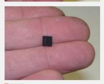
Replace the chip by slicing off the top two corners of melted plastic and sliding the chip out. After replacing the chip if it seems a little loose in the slot, place a dab of hot glue on each of the corners that you sliced off. The hot glue is easily removed when recycling the cartridge again, but will firmly hold the chip in place.
