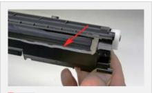
Clean out any remaining toner from the hopper. Note the Dr. Blade seal. It is a sticky substance that can be clean with alcohol if toner gets on it. If this seal becomes damaged, replace it with 100% silicon caulk.
