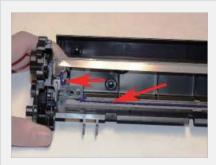
Clean out the waste toner, make sure the seals are clean. If toner gets on the blade seal it can be cleaned with alcohol to activate the adhesive again.
