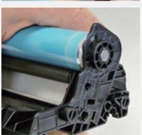
Re-Install the OEM OPC Drum and metal axle pin. The metal axle pin should have a small amount of conductive grease on the tip. Remove the old grease and replace before inserting the pin. Make sure the axle pin is fully inserted.
