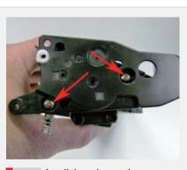
Install the end cap and two screws.
