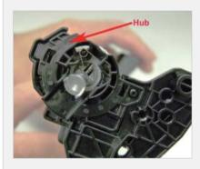
The drum hub on the opposite side is welded. The weld can be broken or drilled out, but there is a good chance that the hub will either warp if pried off, or will be hard to align if drilled out.
