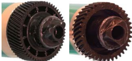
Photosensitive drum with twisted gears
