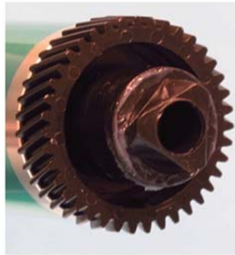
Figure 4. Photosensitive drum with twisted gears
